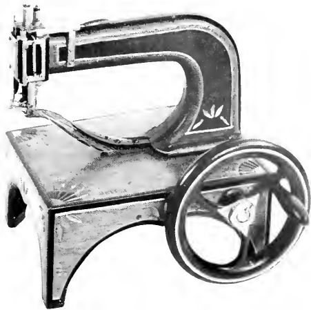
Figure 55.—BLAKE'S LEATHER-STITCHING MACHINE patent model of July 6, 1853; the inventor claimed the arrangement of the mechanism used and an auxiliary arm capable of entering the shoe, which enabled the outer sole to be stitched both to the inner sole and to the upper part of the shoe. (Smithsonian photo 5036L.)
